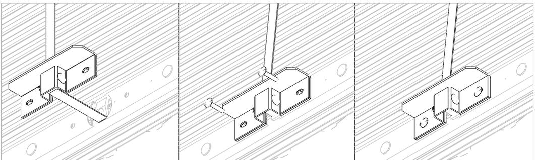
**2** Stretch the strap vertically and place the deck below the seam. Drill diameter 4.2 and put the rivets (be careful to don't damage the front face of the shutter!)
