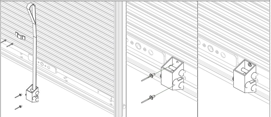
**2** Stretch the strap vertically and place the deck below the seam. Drill diameter 4.2 and put the rivets (be careful to don't damage the front face of the shutter!)
