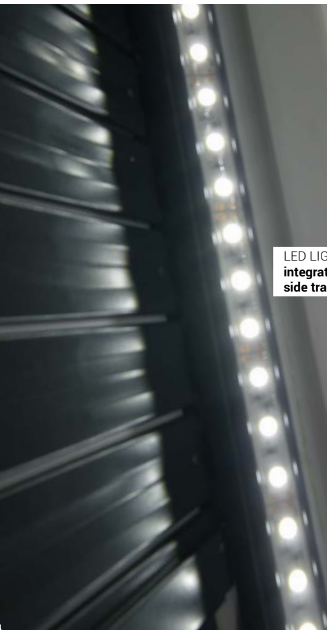
OUTSIDE LIGHTING AREA integrated in a drip channel
